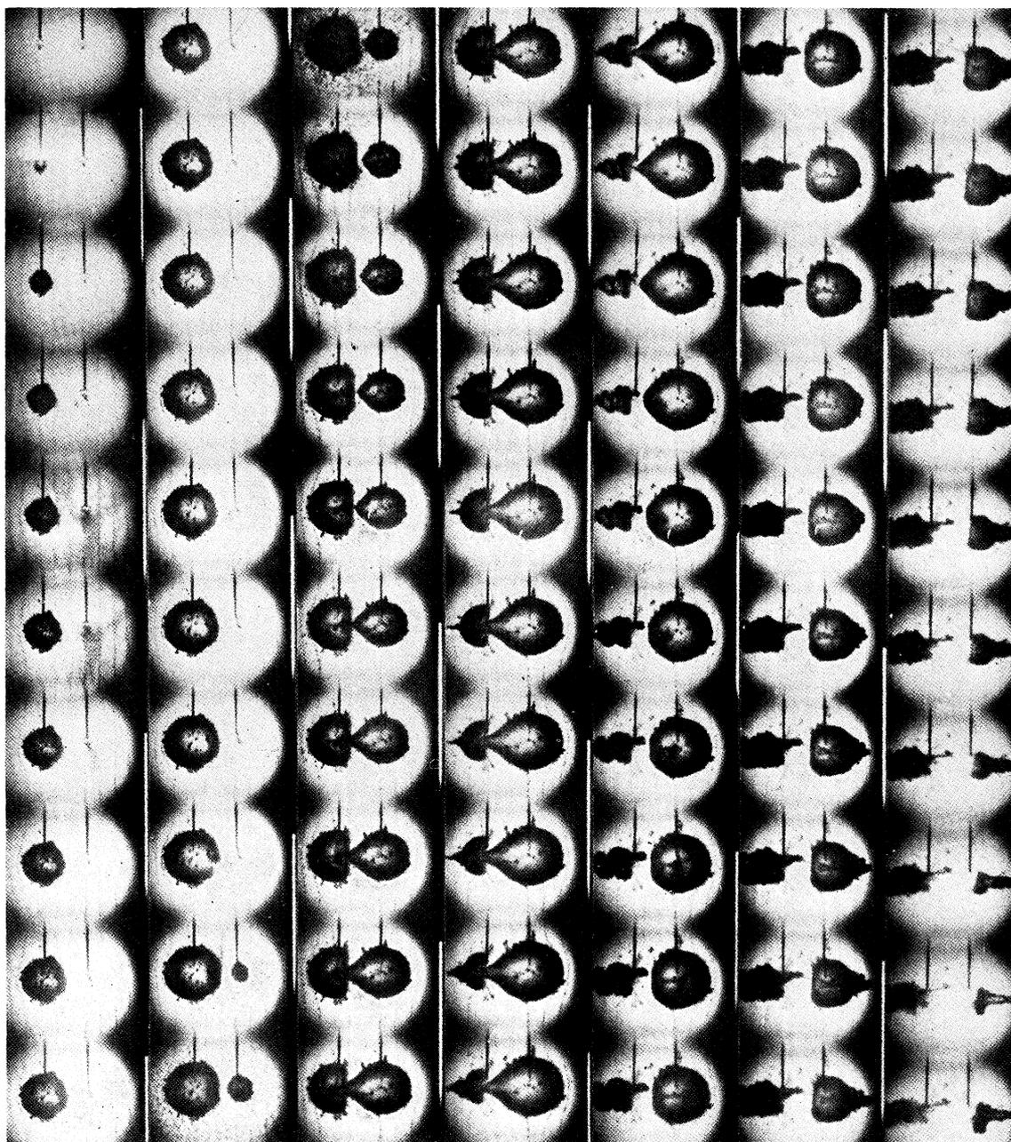
FIGURE 1. Two detonators fired with a time separation of 6 ms (Warren & Price).
