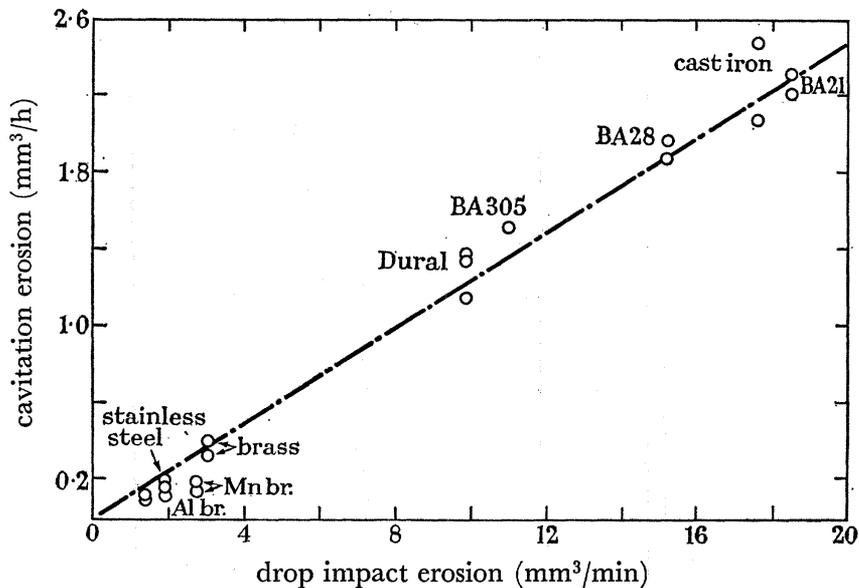
FIGURE 2. Correlation between drop impact and cavitation tests.
