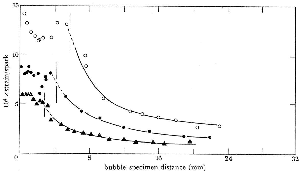
FIGURE 11. Spark energy:  $\circ$ , 4.6 J;  $\bullet$ , 1.0 J;  $\blacktriangle$ , 0.5 J.
