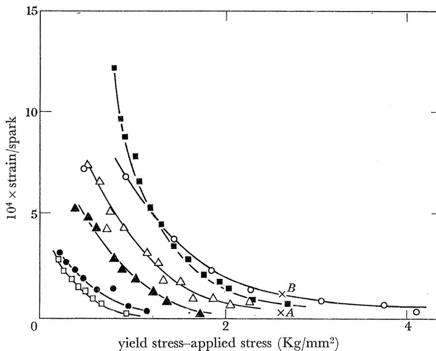
FIGURE 12. Spark energy and separation:  $\circ$ , 1.0 J, 1.48 mm;  $\triangle$ , 1.0 J, 1.5 mm;  $\blacksquare$ , 4.6 J, 1.5 mm;  $\blacktriangle$ , 0.5 J, 1.5 mm;  $\square$ , 4.6 J, 14.2 mm;  $\bullet$ , 1.0 J, 5.7 mm.
