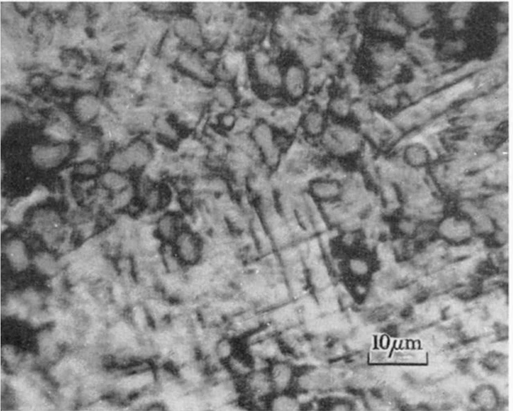
FIGURE 9. Cavitation damage on surface of specimen after magnetostriction testing.
