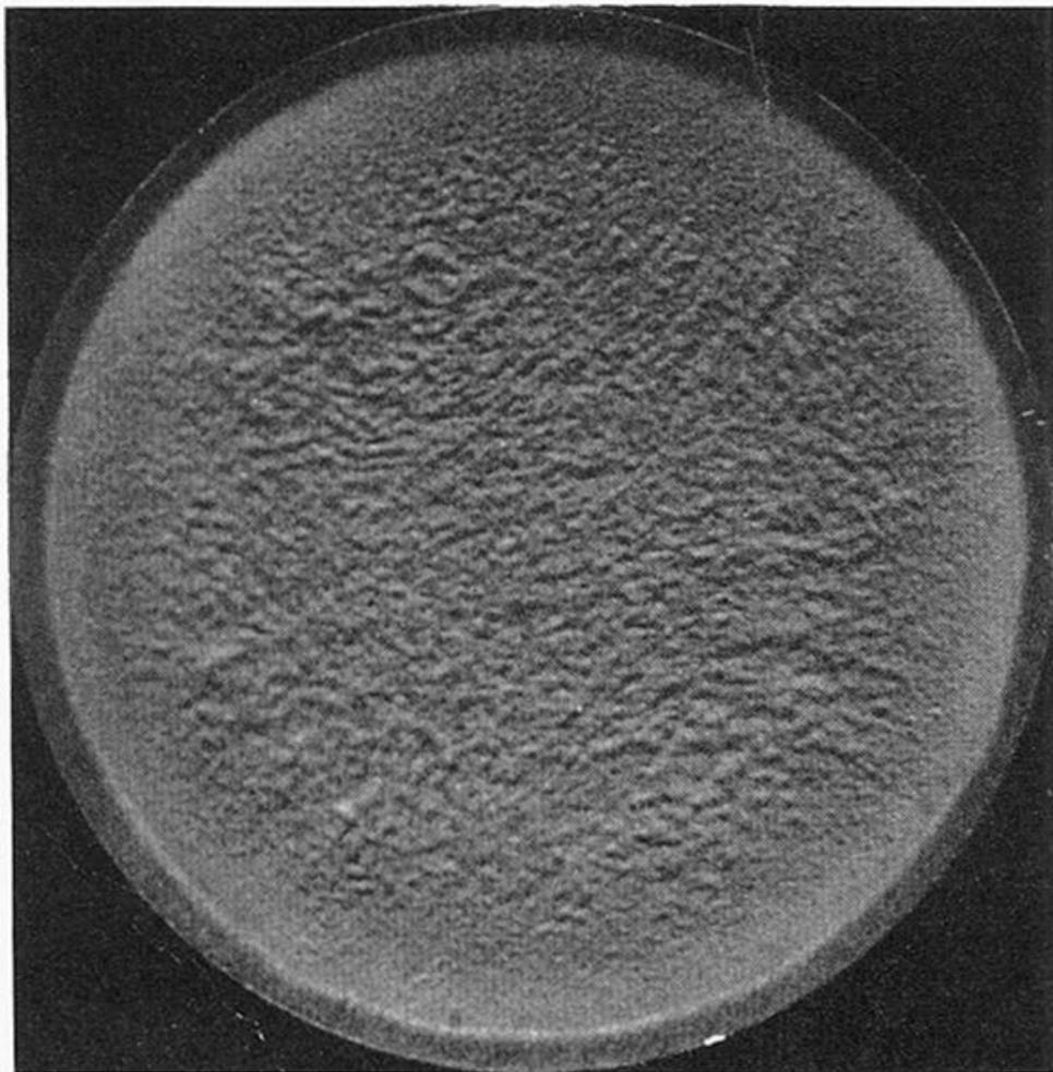
FIGURE 5. A wrought nickel-aluminium-bronze specimen after 10 h test.
