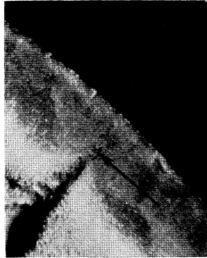
FIGURE 4. A typical pore (arrowed) at the tip of a rut.
