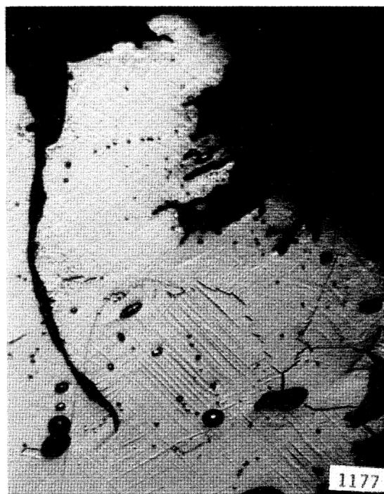
FIGURE 8. Section of type 316 stainless steel impellor in area of heavy cavitation damage from mercury. (Magn.  $\times 800$ .)
