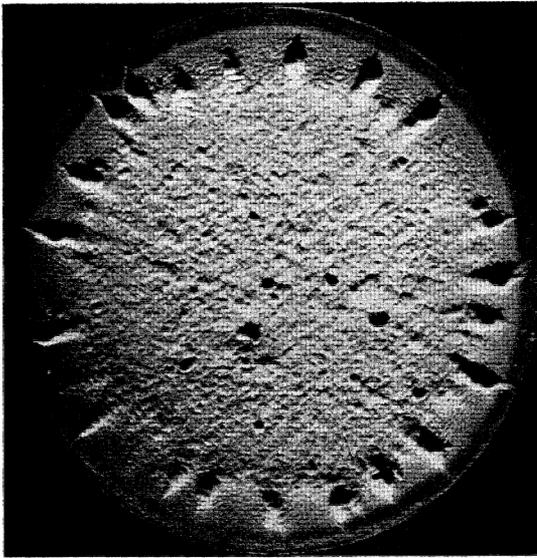
FIGURE 3. A cast nickel-aluminium-bronze specimen after 10 h test.
