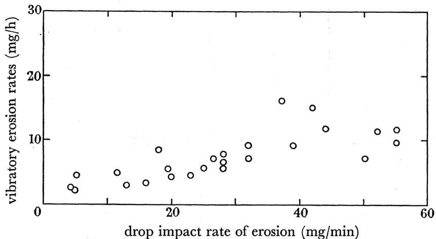
FIGURE 3. Correlation between impact and vibratory tests.
