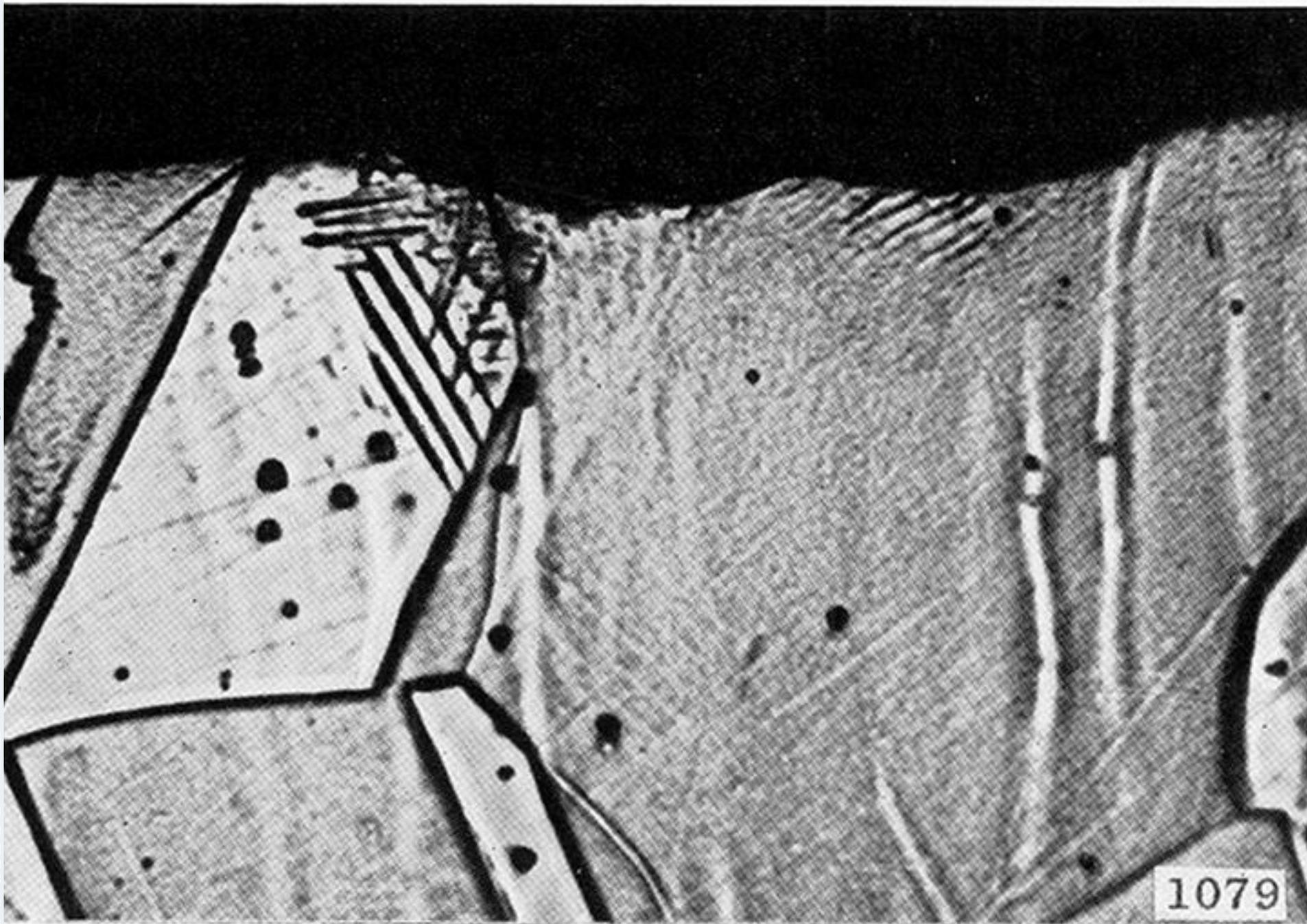
FIGURE 7. Typical section through an irregular shaped pit on stainless steel sample no. 26-3 (which had been run for 11 h at 'standard cavitation' at a throat velocity of 95 ft./s in water), showing slip lines. (Magn.  $\times 800$ .)
