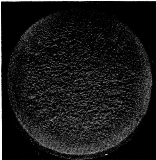
FIGURE 5. A wrought nickel-aluminium-bronze specimen after 10 h test.
