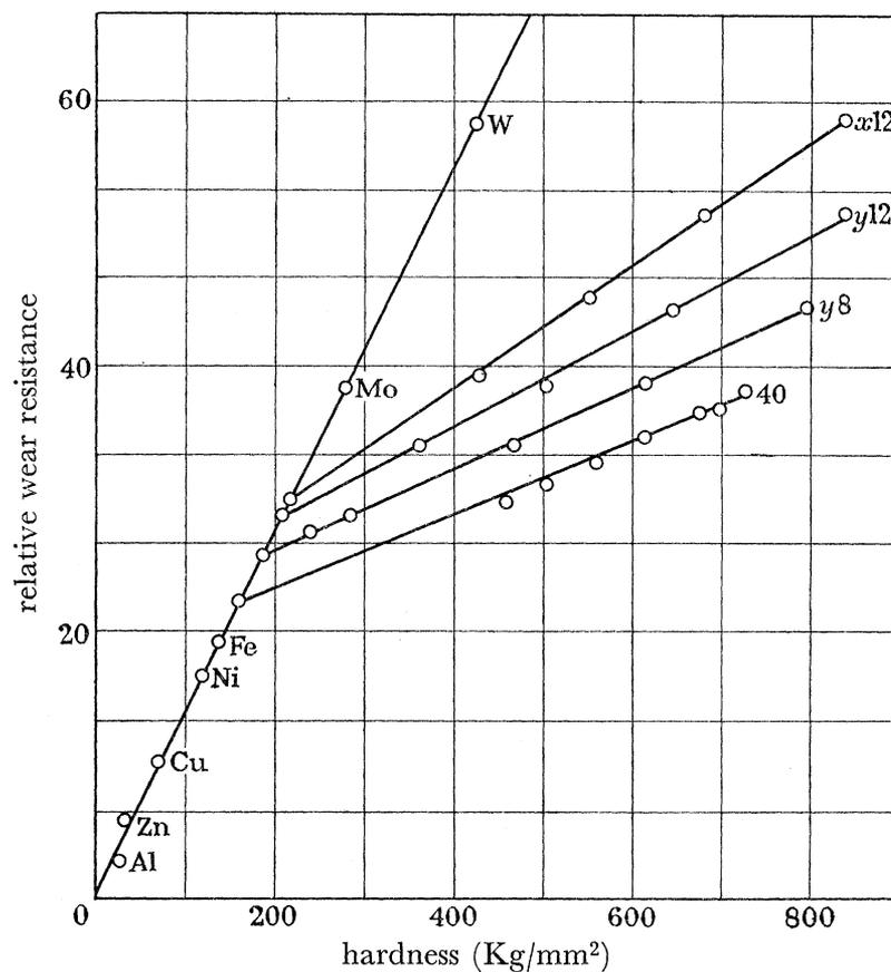
FIGURE 10. Wear resistance of pure metals and steels as a function of indentation hardness (from Khrushov 1957). The steels are indicated as follows: 40, carbon 0.41%; y8, carbon 0.83%; y12, carbon 1.10%; x12, carbon 2.35%; chromium 11.9%.
